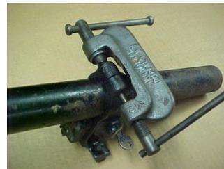
Pictured above is the special KR Wilson tool number BV12. This tool is designed to remove the tamper resistant bolt from the column lock housing. The tool has two threaded shafts in a C frame.
