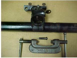
Pictured above is the bolt removed from the lock housing and the housing then removed from the steering column tube.
