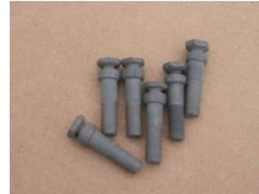
Pictured above are NOS B-3731 twist-off head screws used to secure the steering column ignition lock to the steering column. These screws are tightened until the hex head twists off, leaving a flush, smooth, round, and tamper-resistant bolt.
